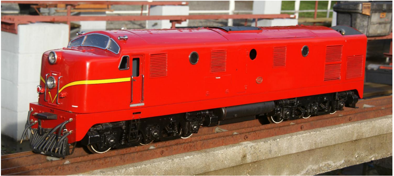
Two great 3.5" gauge diesel models, petrol powered Dg 785 (top) and battery powered Dc 4352.
