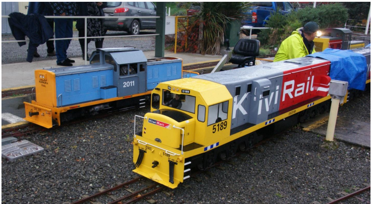
MU cables and controllers being set up on Tony Winter's double heading Dxc's with other diesels being prepared to run on the track behind.
